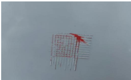
Paint adhesion level 1
